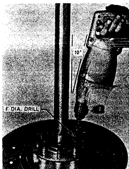
Fig. 326—If special axle puller (Figs. 323, 324 & 325) is not available, drill through collar with \frac{3}{8} -inch drill, then enlarge hole with \frac{1}{2} -inch drill as shown. Drill will speed up when it contacts bearing cone.
