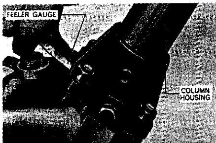
Fig. 25—Measuring clearance between gear housing and steering column housing to determine shim and gasket thickness needed. Shim and gasket thickness required between gear housing and side cover is determined in similar manner.
