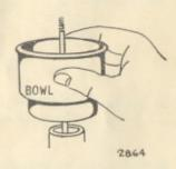
1. Remove Wing Nut 2. Lift Out Element
